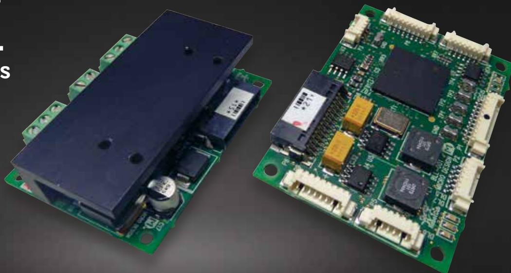
This motor controller is made of two separate boards. The BLL contains the logic circuits, while the BLP includes the power drivers. The controller is capable of driving up to two 250W Brushless DC motors using CAN bus communication for command and control data exchange.
