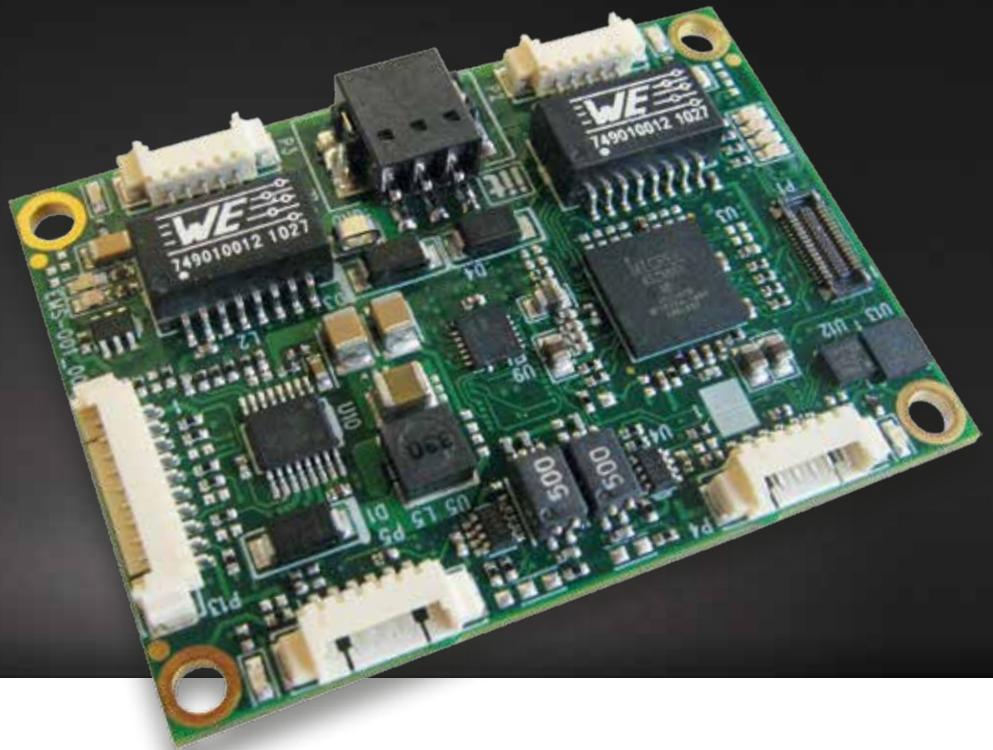
The EMS4 card is a 32-bit Arm Cortex-M4 embedded microcontroller based device designed for managing several communication channels in robotic applications. Its main function is to provide the bridges among two Ethernet 10/100 base-T high-speed link, two CAN-2.0B buses and six SPI-master buses. When connected to external motor-driver cards (i.e. 2FOC, BLL/BLP or MCP/MC4), the EMS4 embedded microcontroller provides enough computational power to directly manage up to four motor control-loops.
